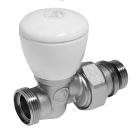
Straight manual valve, with connection for copper, plastic or multilayer pipe adaptor. Fluid of use: water and glycol solutions (max. 30 %) Temperature range: 5÷110 °C Max. working pressure: 16 bar
